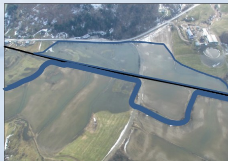
Excavating abandoned railroad bed (in black), restoring floodplain
