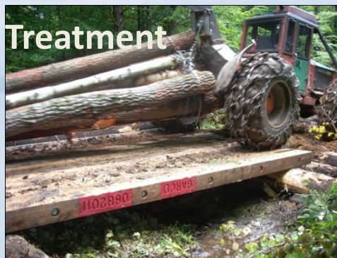
Portable skidder bridge protects water quality during timber harvesting operation
