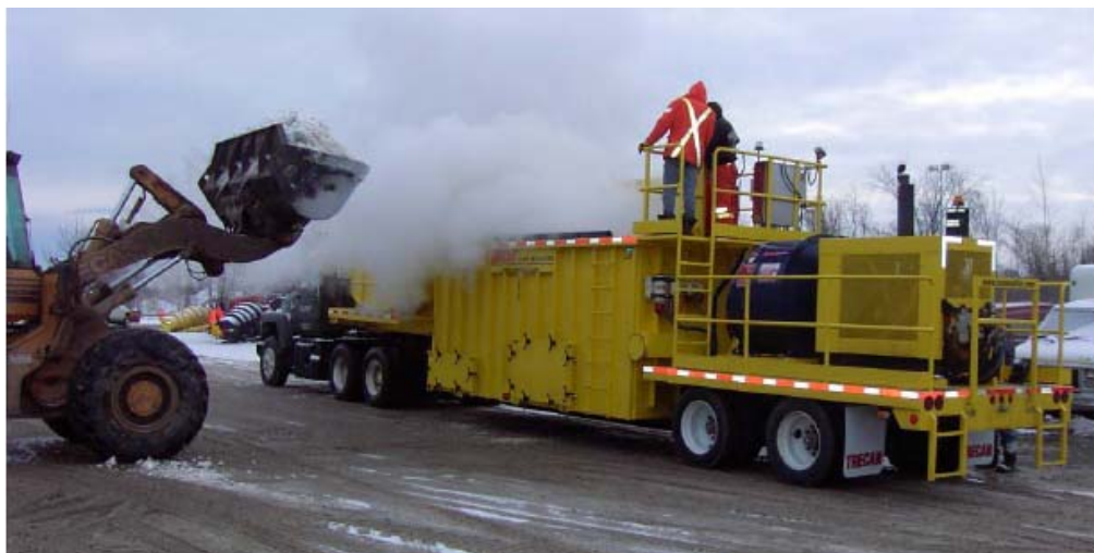
Trailer type snow melting machine in action (Snowmelter 2005)
