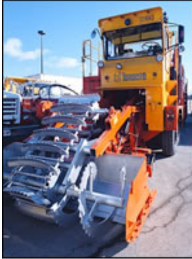
Self Propelled, self feeding snowmelter (City of Toronto 2005)
