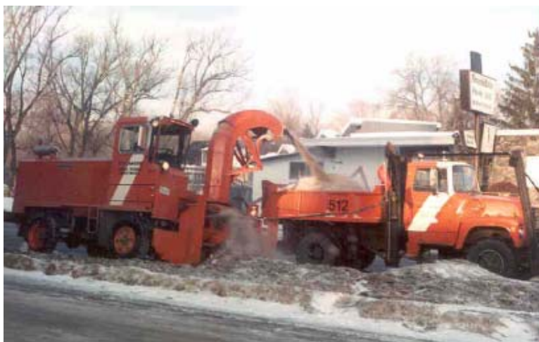
Using a snow blower to load trucks of hauling contaminated snow banks ( http://www.ogra.org/lib/db2file.asp?fileid=9198 )
