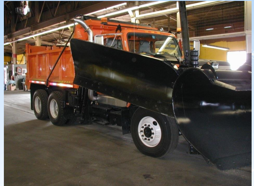
Category 16 Truck with right-hand wing plow and right-hand fixed -angle front plow
