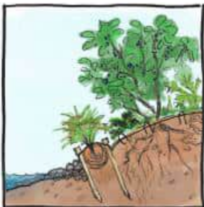
Regrade and slope back, install erosion control blanket, fiber log, & rock toe.
