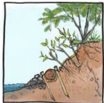
Leave & patch with erosion control blankets, fiber logs, & stone toe. Plant live stakes.
