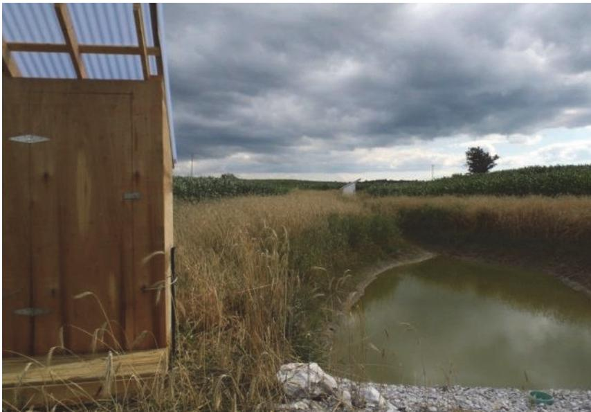
developed for the WASCoB illustrates that when the water level rises above the top orifice of the standpipe and again when the spillway is overtopped, a modest 1-cm increase in stage corresponds with a 30 percent increase in flow rate. Therefore, relatively small errors in stage measurement due to sensor drift or movement or small waves on the pond may translate to large errors when computing flow rates based on a stage-discharge relationship.
