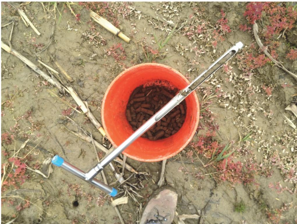
**Figure 2.** Soil probe used to collect composite soil samples
