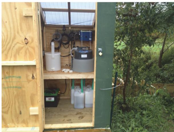
Figure 5. Instrument shelter with autosampler and carboys
