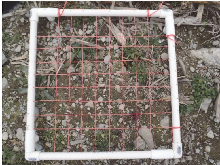
Figure 3. Quadrat used in cover crop percent cover measurements
