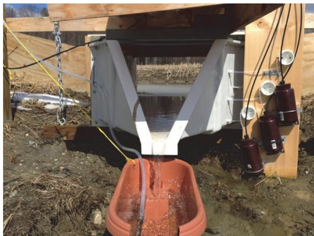
Figure 5. H-flume, splash pan, and siphon sampler array
