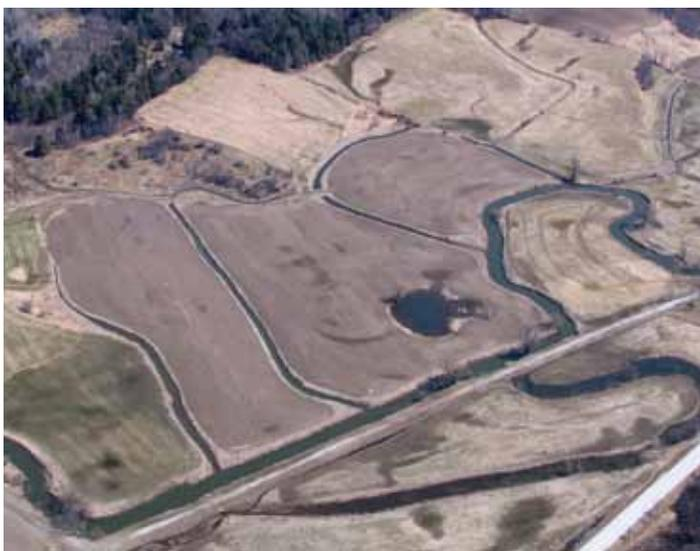
*Construction of the Lamoille Valley Railroad along this reach of Black Creek in Fairfield required about six miles of embankment (bringing in soil fill) that destroyed about 200 acres of functioning floodplain and wetlands.*
