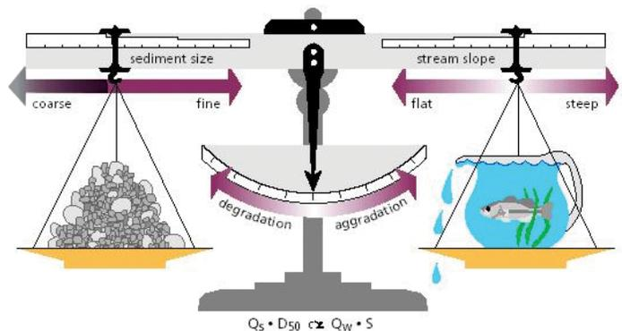
Lane's Balance of Sediment Supply & Sediment Size with Slope & Discharge (Lane, E.W. 1955. *The Importance of Fluvial Morphology in Hydraulic Engineering*. In *Proceedings of the American Society of Civil Engineers* 81(745): 1-17.) Reproduced by permission of the American Society of Civil Engineers.
